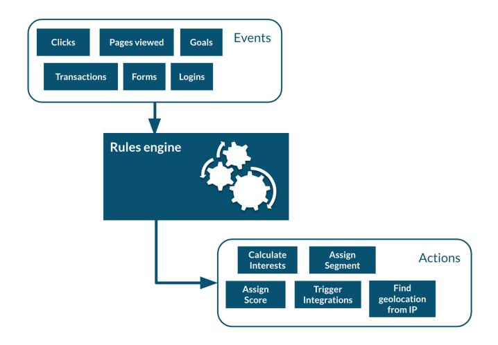
Apache Unomi has a built-in rule engine that is one of the most important components of its architecture. Every time an event is received by the server, it is evaluated against all the rules and the ones matching the incoming event will be executed. You can think of a rule as a structure that looks like this:
