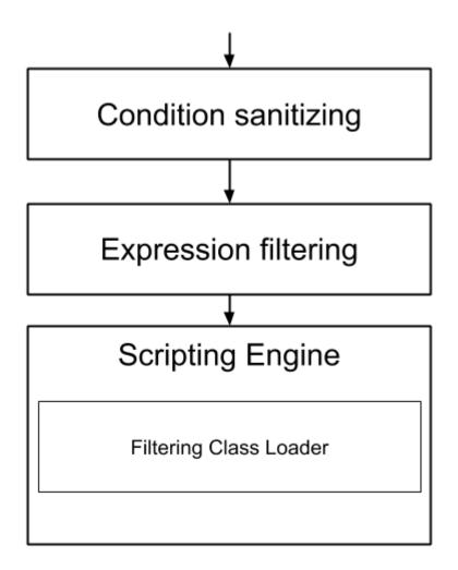
Conditions submitted through the context.json public endpoint are first sanitized, meaning that any scripting directly injected is removed. However, as conditions can use sub conditions that include scripting, only the first directly injected layer of scripts are removed.
